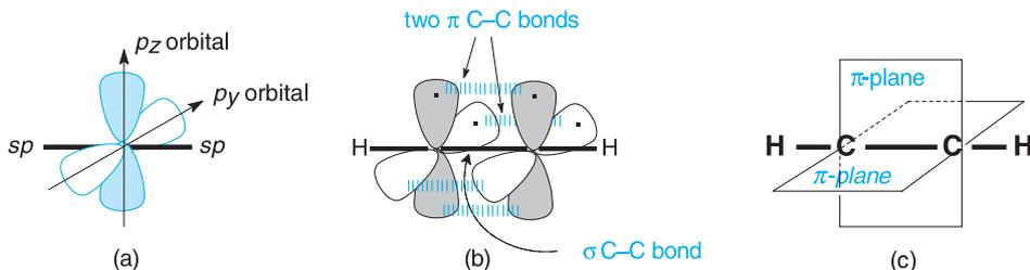
**Figure 1.9.** The  $sp$ -hybridized carbon (a), the schematic orbital formula of acetylene (b), and two mutually perpendicular  $\pi$  planes that formed two  $\pi$  bonds. The orbitals involved in the C–H and C–C single bonds are omitted for clarity.
